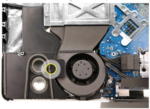
2. Disconnect the speaker from the audio board. The speaker cable runs under the black plastic cable guide (above the memory slot) and connects to the audio board on the right side of the logic board.
